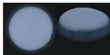
Fiber endface pre-melted after
